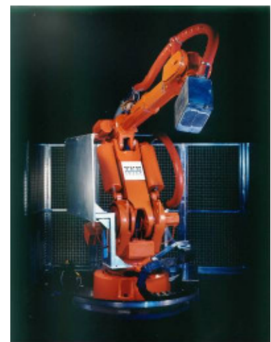
Dot Paint Marking Machine Robot Version
